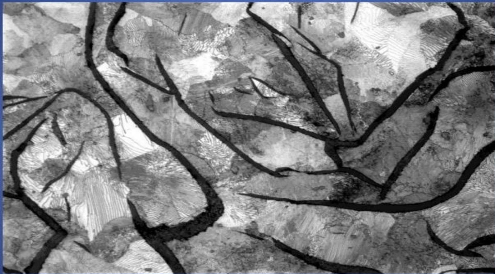
Gray cast iron microstructure
