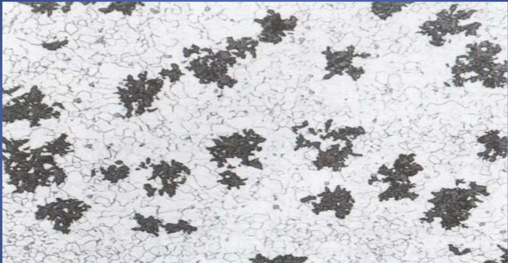
Malleable Cast Iron Microstructure
