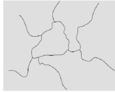
(d) The grain structure as it would appear under the microscope; dark lines are the grain boundaries.
