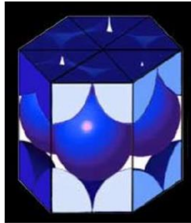
Figure 1.3 The hexagonal closed-packed lattice structure
