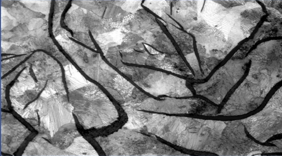
Gray cast iron microstructure
