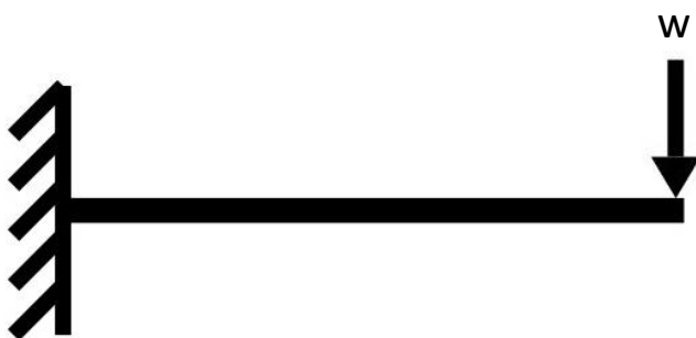
Cantilever beam with concentrated load w .
