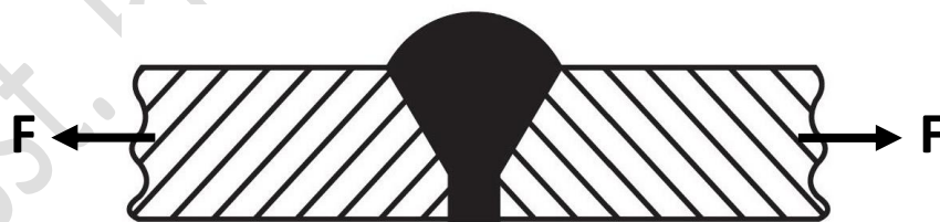
Single V-Butt weld joint
