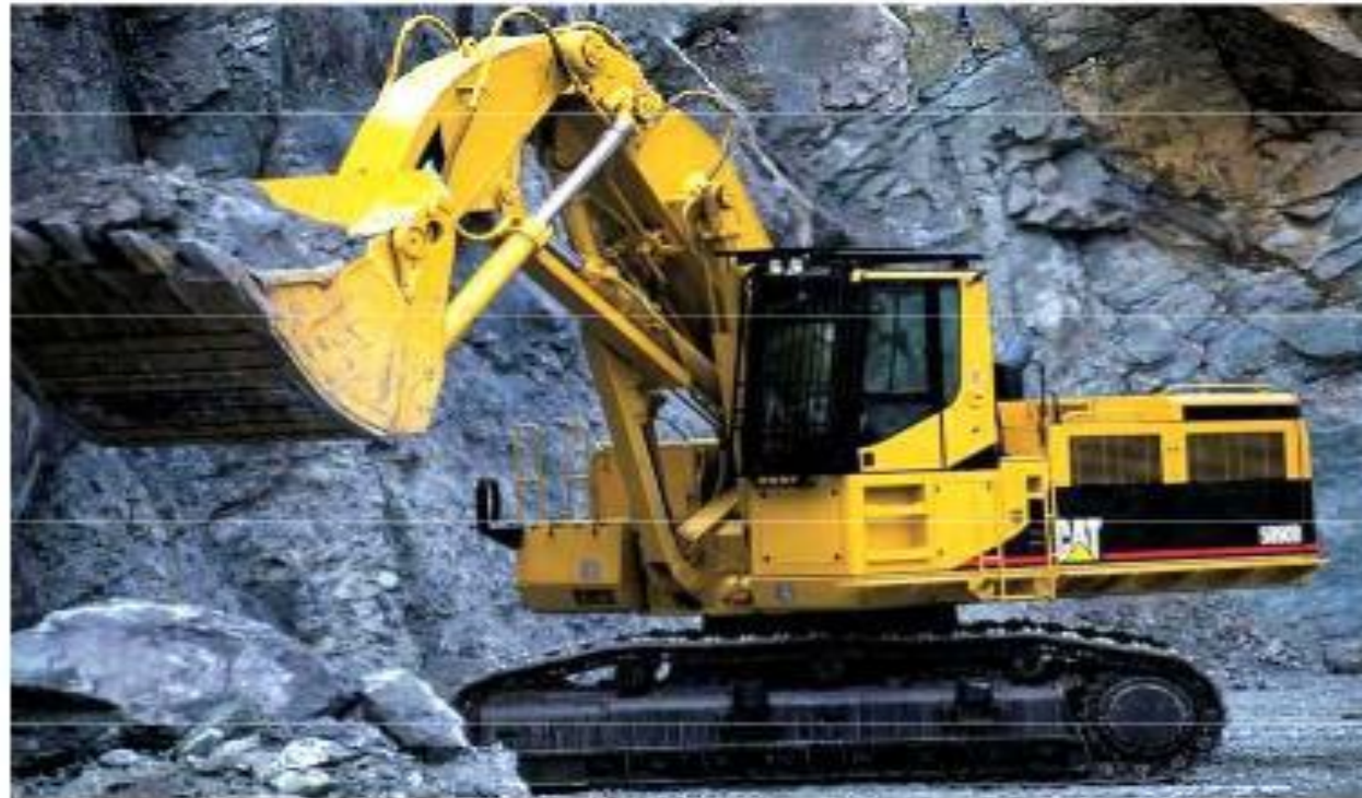
Front shovel, track-mounted
