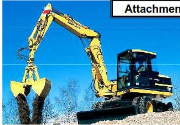
Clamshell bucket (for granular material)
