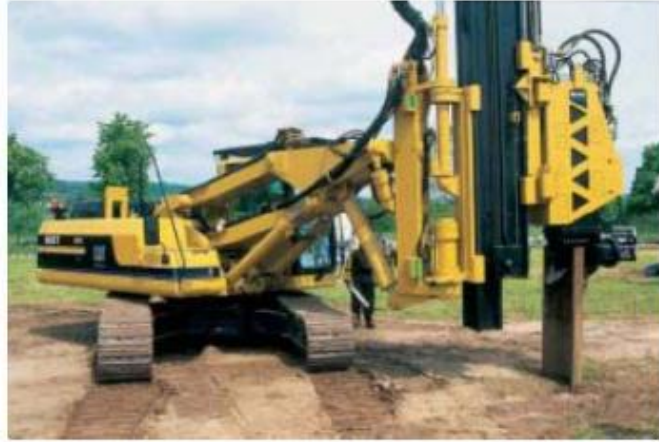
Sheet-wall piling equipment
