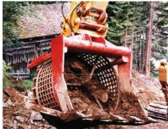
Screening adapter (for recycled material)
