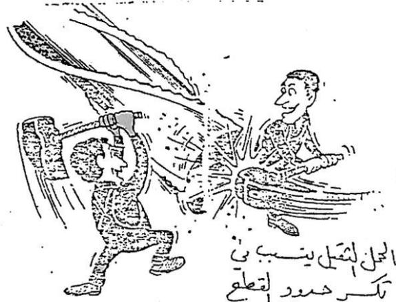
Fig. 57-5 Too heavy a load on the cutting edge will cause it to chip. (Courtesy The Weldon Tool Company)
